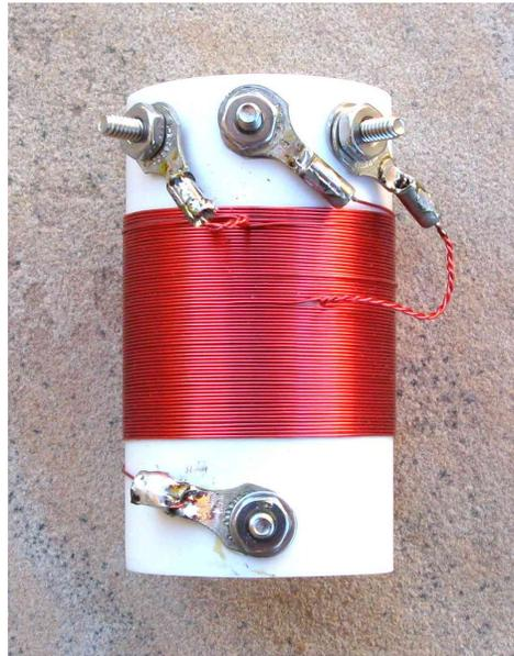
*We have found that when heat is applied, soldering the ring terminals, it may cause the 4-40 hardware to loosen. Go back over the four 4-40 nuts and tighten the connections after soldering. Hold on to the ring terminal sleeve so it does not rotate during this process and break the magnet wire.*
