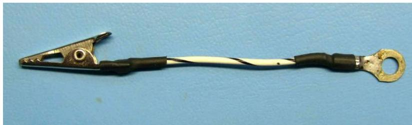
Attach the clip assembly to the upper coil end post with a 4-40 nut, and secure.
