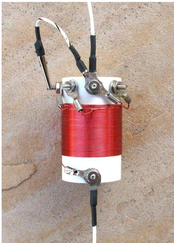
For storage, just disconnect the radial wires. Leave the element wires and loading coil attached. Place the loading coil inside the base pcb cutout. Wrap the upper element wire on one side and the lower element wire on the other side. Secure the assembly with the rubber bands you used to attach the base pcb to the fiberglass mast.
