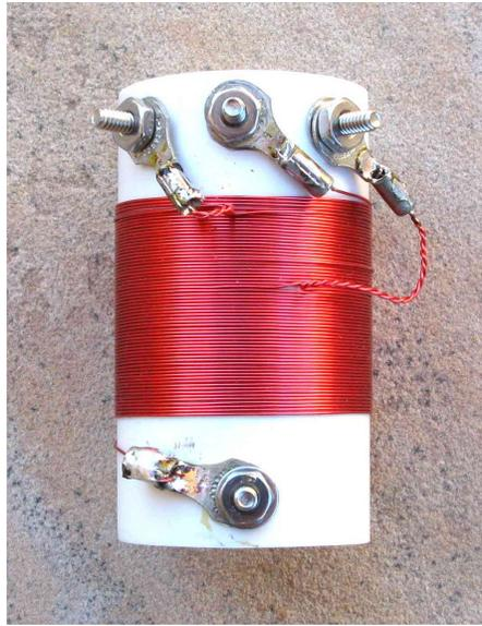
Print this page and scale your printer if necessary to achieve the 2.25" dimension shown. Cut out the rectangle and tape it to the  $\text{\O}1$ " PVC pipe coil form, centered on the length. If the coil form is not 2.25" long, trim down by sanding to length, or it might not fit in the base cutout.
