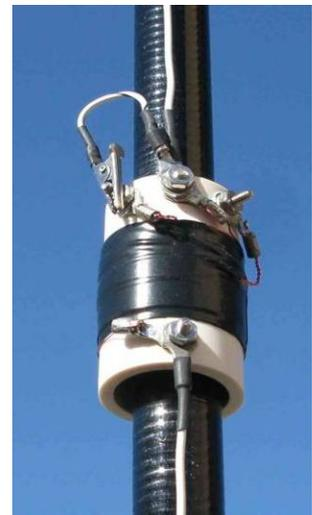
Strip, tin, and route the 7.5' lower element wire through the base pcb as shown below.
